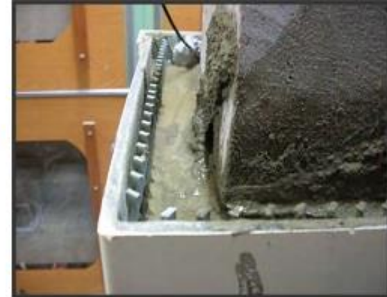
Grout with Conductive Mortar
